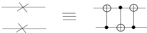
Fig. 18. Swap gate implementation using basic gate.
